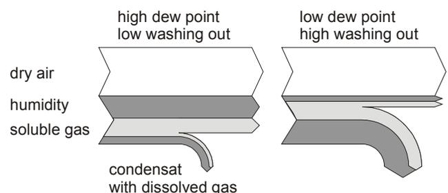
Figure 2: Diagram of condensation and absorption caused by dew point reduction
