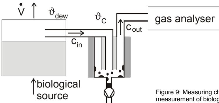
Figure 9: Measuring chain for the measurement of biological emissions
