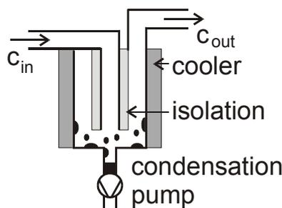
Figure 1: Principle diagram of a measuring gas cooler for dew point reduction
