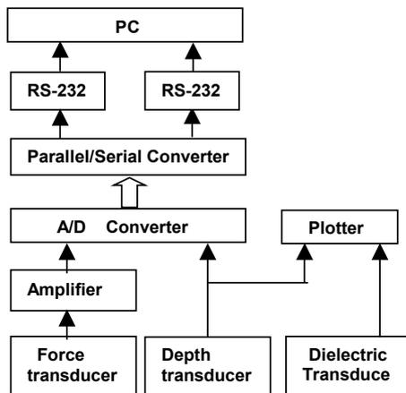
Figure 4: Block diagram of the experimental measurement system
