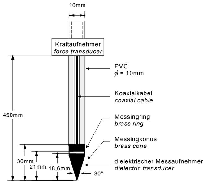
Figure 1: Schematic diagram of the dual sensor
