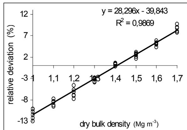
Figure 6: Relative deviation of the output of the dielectric transducer versus dry bulk density
