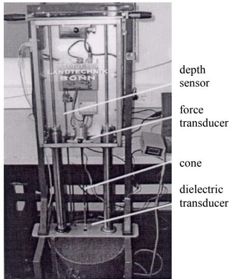
Figure 3: The experiment system of the dual sensor
