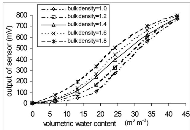
Figure 5: Signal of the dielectric transducer versus volumetric water content depending on different bulk densities
