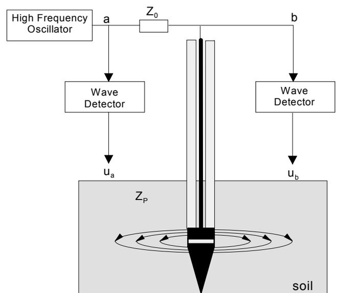
Figure 2: Schematic diagram of the dielectric transducer
