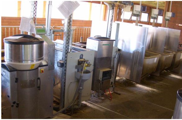
Fig. 2: System set-up (from left to right): milk feeding robot, feeding station with temperature measuring system and animal weighing system, concentrate feeding robot, drinking water robot and separated roughage weighing troughs
