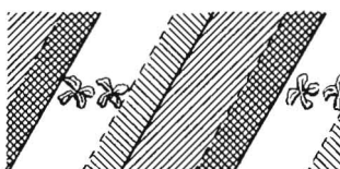
Abb. 12: Parallelschlag Messerkombination 8 x 1\frac{3}{4} " + 16 x \frac{5}{8} "
